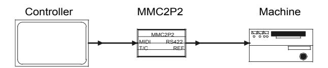
The MMC2P2 Interface uses experience gained from both the SR and MR series remote control system. Designed to be used with existing consoles and DAW's the interface will connect any MMC Midi Output and MTC Midi Input to a RS422 P2 Protocol serial port on any machine.
