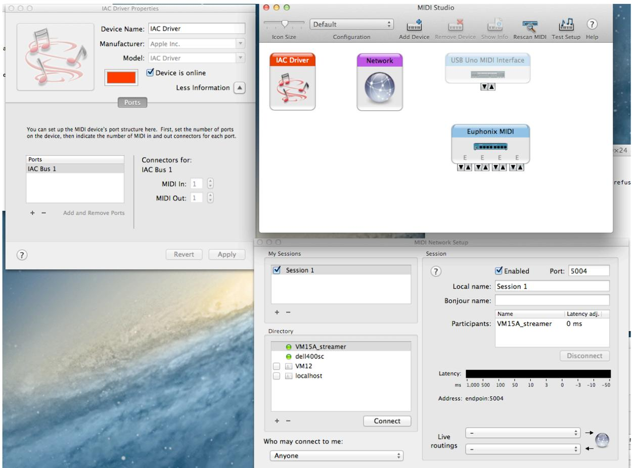
Open Protools. Go to the Setup/Peripherals menu item. Select IAC Bus 1 as the MTC output port.
