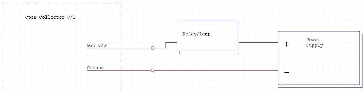
Connecting a LED to a Open Collector Output
