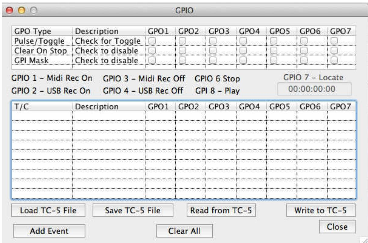
By default all GPO's are cleared on stop, the Clear On Stop Mask can be used to disable this. The GPO's pulse for about 100mSec and can be selected to Toggle.
