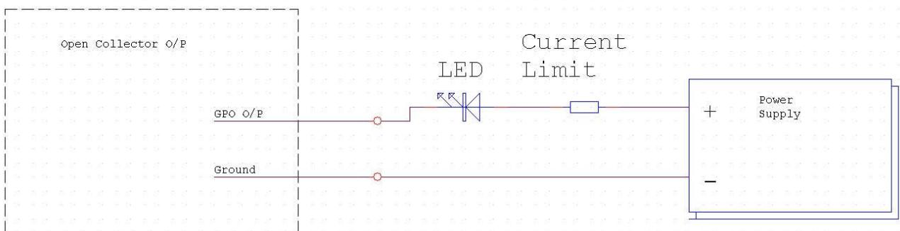
The Current Limit resistor can be calculated typically 330R for a 5v Supply and 1K for a 12v Supply.
