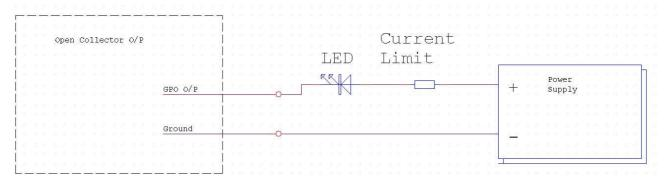
The Current Limit resistor can be calculated typically 330R for a 5v Supply and 1K for a 12v Supply.
