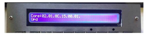
Programming Screen after enable and file selection. The firmware files can be posted as a zip file, if they are extract the .bin file before use.
