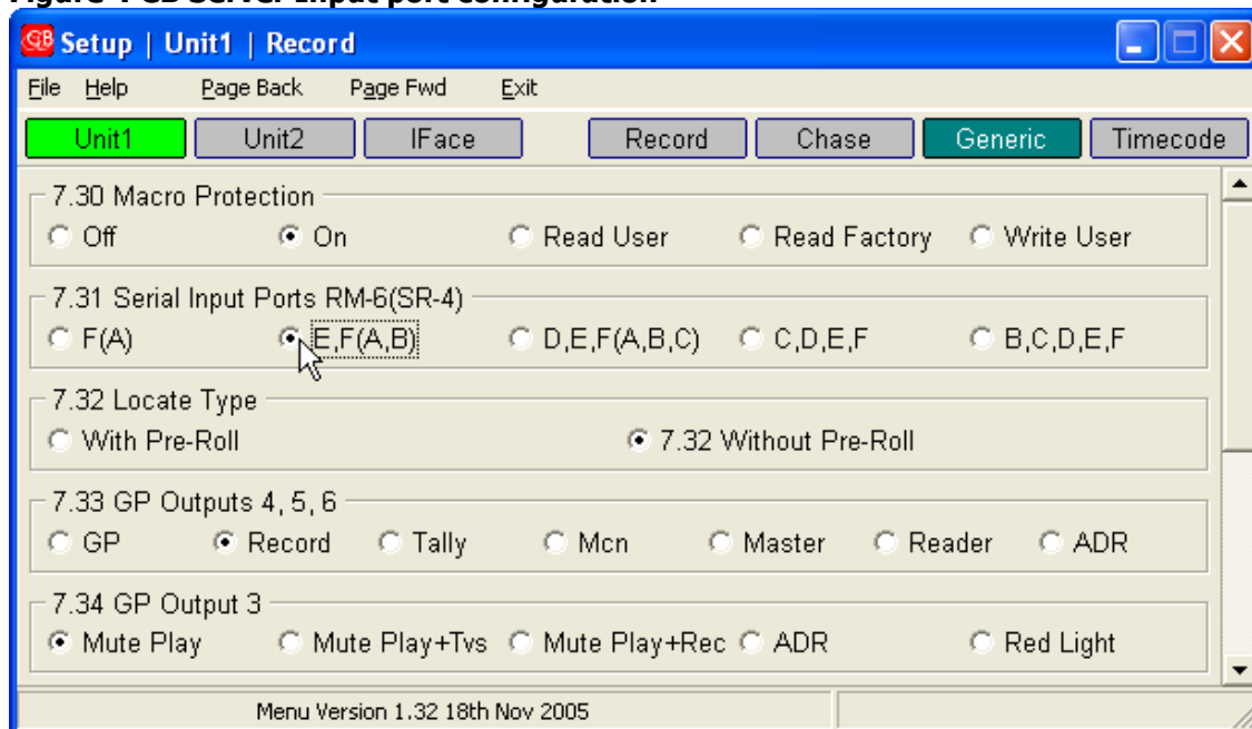
Figure 4 CB Server Input port configuration
