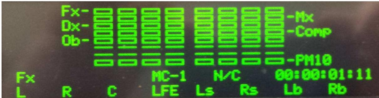
Stem Track Arm Display: Stems 1-8 displayed in 8 track mode, Note1. The names are on alternate sides
