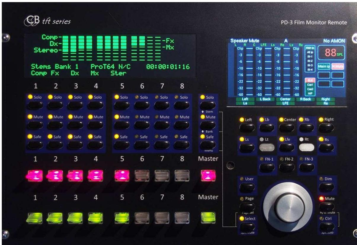
The PD-3 showing the new O-Led Display which includes a display of the stem track Arm status, set to display 12 tracks, Note Comp, Fx and Dx all have 10 channels assigned, Mx has 8 channels assigned and Stereo has two channels Assigned, All assigned tracks are in record.
