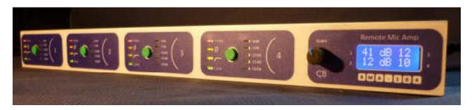
The MA-104 is a high quality microphone preamp with remote control via Ethernet or Midi over USB(Pro Tools 'Pre' Protocol). It is a low noise four channel amplifier with balanced Mic/line input and two line outputs.
