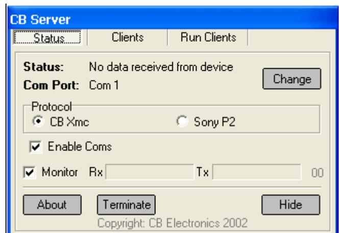
**Protocol:** the CB Server may be setup for Xmc multi-machine protocol or standard Sony P2 Protocol.
