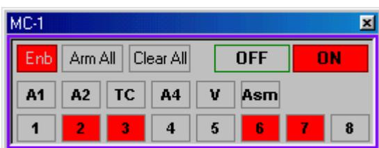
The track-arming window includes Record Enable, track arming and record on/off as 'Illuminated Switches'.
