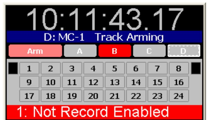
keyboard or on the Master Display software to select the machine or system arming display and control. The Track arm display is combined with a machine select panel. The following information is displayed:
